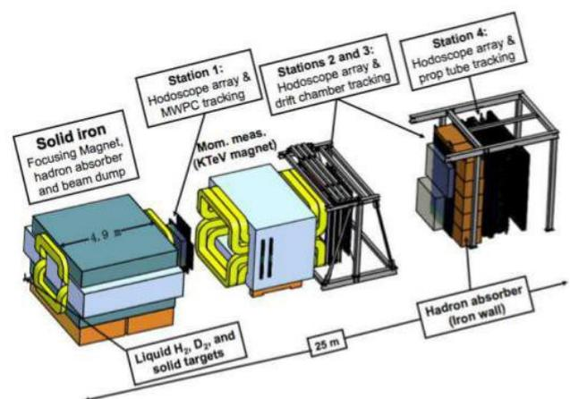
There is a magnet and drift chambers for tracking and momentum determination of charged particles. Hodoscopes are used as triggers for the drift chambers.
